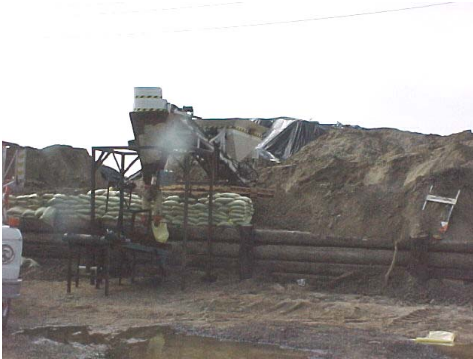
Companies that provide ready made sandbags have hopper and conveyor belt production and can turn out thousands of bags in a short time
