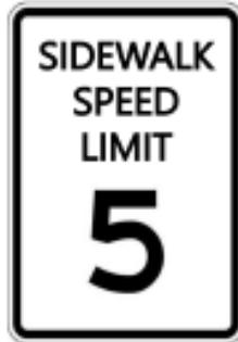
Figure 4.7 Sidewalk Speed Limit Sign (Modified R2-1 )
